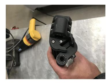
3. Use the hardware from the "U" brackets to mount your light onto the Shock Tower Bracket.
