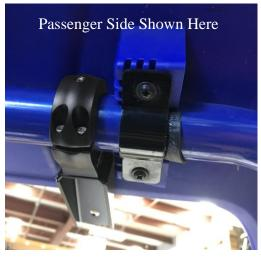
4. Detach "U" bracket from two bottom mounts and replace the pre-existing bolt with the given M8 x 16mm bolt (keep nut and washers for Step 8). Reinstall the "U" bracket onto the bottom mounts.
